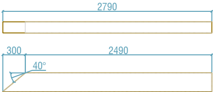
Pilares - Chapa dobrada 250x150 #2.65mm
